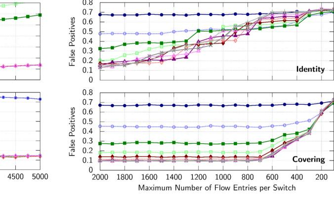
subscribe with OpenFlow combines efficiency and flexibility. Publishers encode matching subscriptions as Bloom filters in the IPv6 source and destination address so that the network switches can derive forwarding decisions using standard OpenFlow bit vector operations only. Furthermore, we developed and evaluated strategies to effectively limit the number of falsely delivered notifications as well as to deal with the switches' restricted capacity to store forwarding rules.
